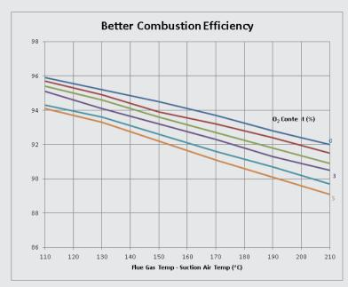
The O2 trim control system provides continuous adjustment of the fuel to air ratio by constantly monitoring the O2 levels in the exhaust gas, resulting in additional fuel savings.
